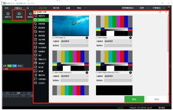
4. Click the 7105 video in video device, click the setting icon behind the device model, an audio and video parameter setting window will appear; select YUV2 as the video format, and the maximum video size is 1360X768; the video format is MJPG, the maximum video size is 1280X720; built-in audio Select digital audio interface (2-7105 audio in), click OK after setting; as shown below
