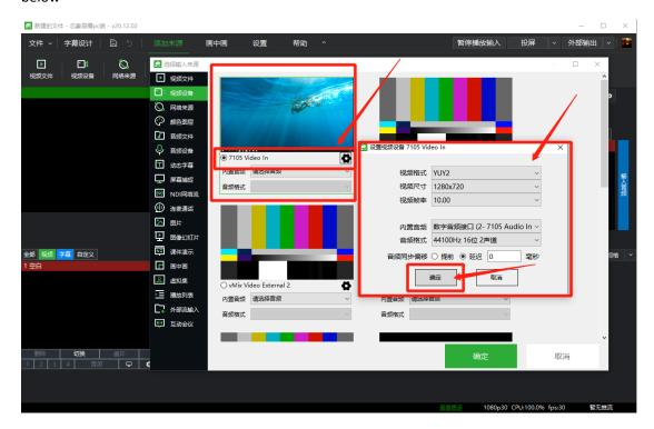
5. The built-in audio and audio format under the device model map the parameters just set, click OK; as shown below
